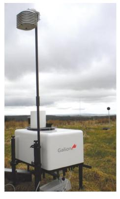
Compact, portable, robust and discreet, the Galion Lidar can be deployed very quickly and provides a much more economical overall NIA solution when compared to traditional met mast methods.
